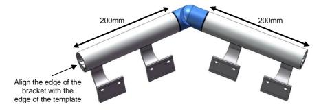
2. Set up a laser level to ensure that the brackets will be mounted horizontally. Align the template with a mark on the wall which has been set for the prescribed handrail height. Draw a line at the end of each bracket as in the sketch below and mark the hole centres for the outer brackets.
